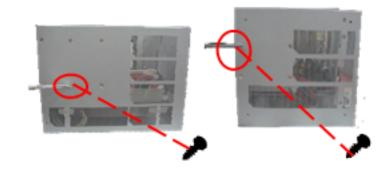
Step 7 Close the top cover back to the chassis and fasten all screws.
